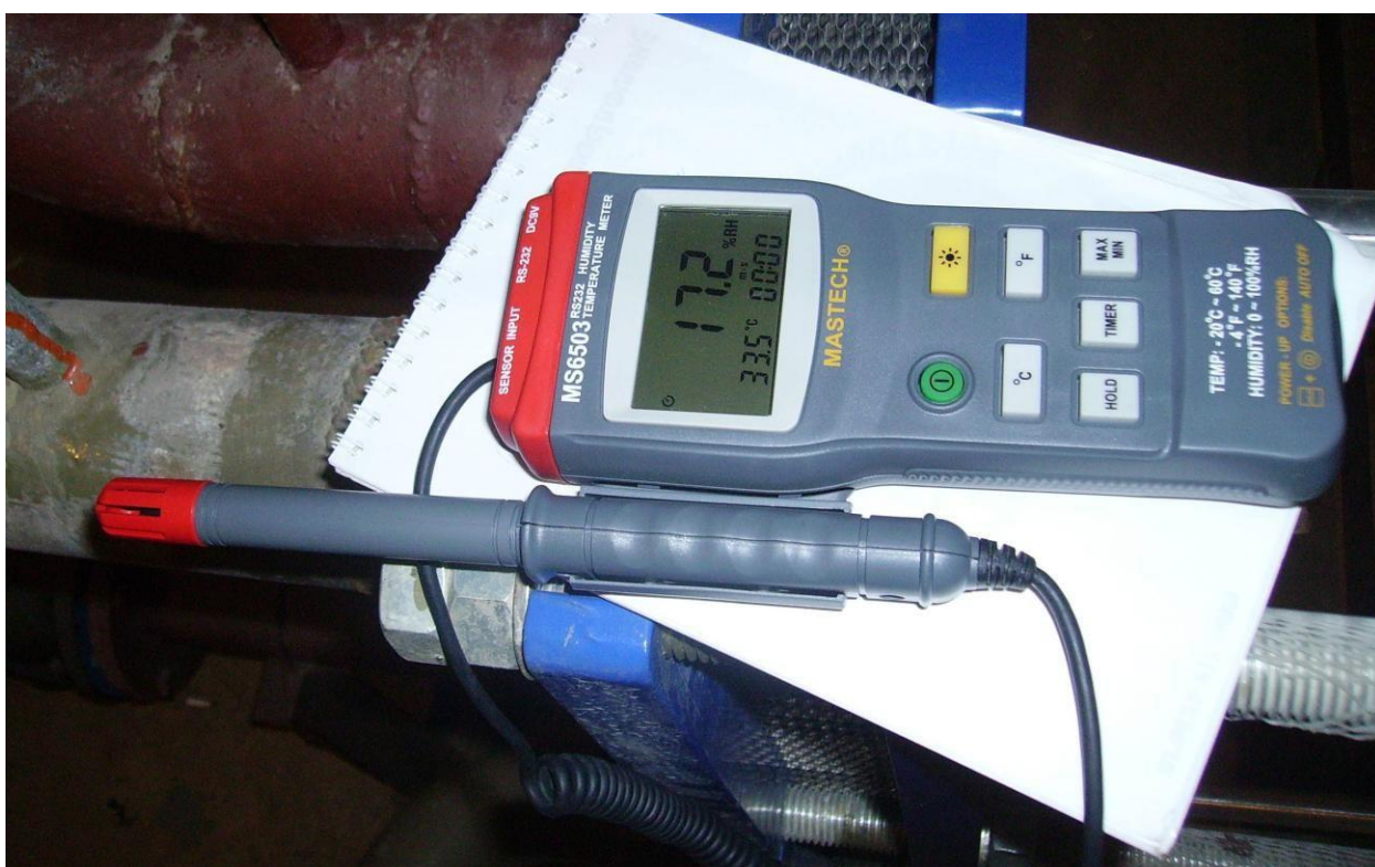
Fig. 5. Contact measurement of the pipe surface.
