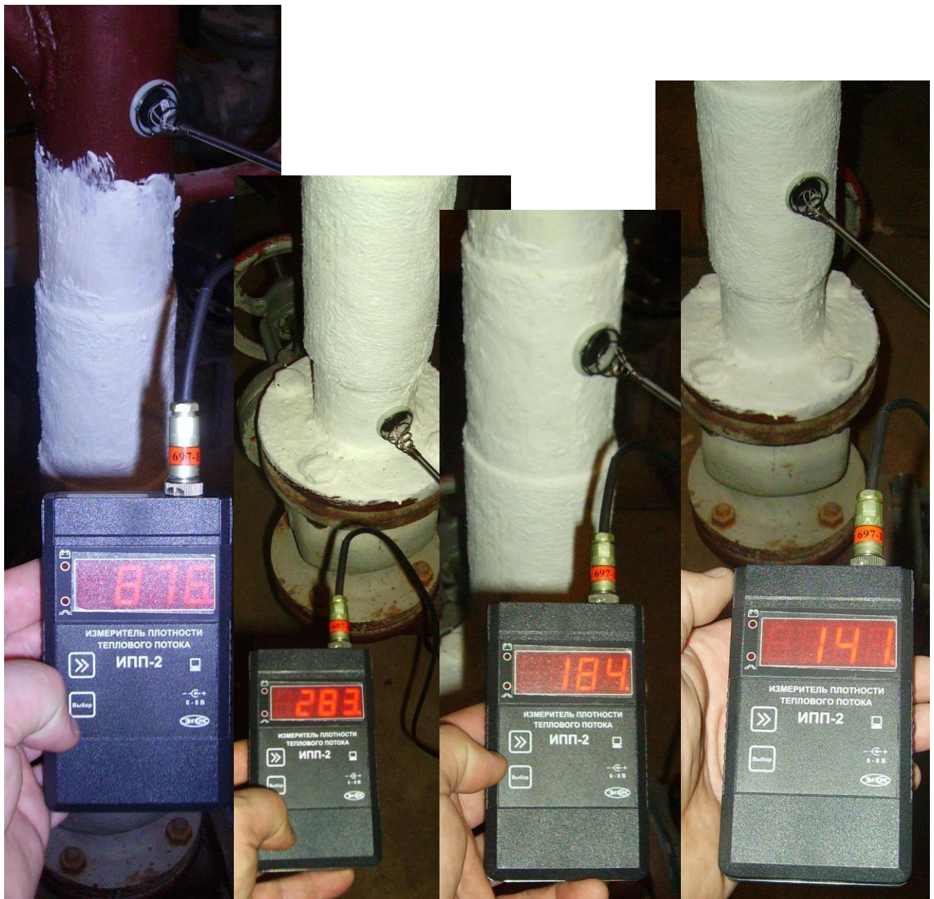
Fig. 3. Measuring heat flux from the surface of the pipe.
