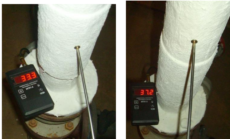
Fig. 5. Contact measurement of the pipe surface.
